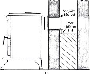
steel sheet or concrete. A short length of flue pipe no smaller in diameter then the stove flue outlet or the manufacturer's stated flue size may then be used to connect the stove to the chimney. This flue pipe should be of cast iron, 316 grade stainless steel or vitreous enamelled, nominal thickness 1.2mm. Ensure that the pipe end is no closer than 76mm to the side or rear chimney walls.
